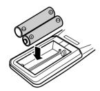
(2) Load the batteries. Insert two R6P(SUM-3)/AA(15F) batteries. Match the polarity (+ and -) of the batteries with the + and - marks inside the battery compartment.
